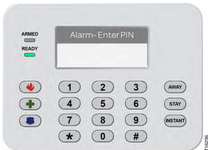
Figure 114: Keypad (Model SR-KPD02)—FIRE (Alarm- Enter PIN)
