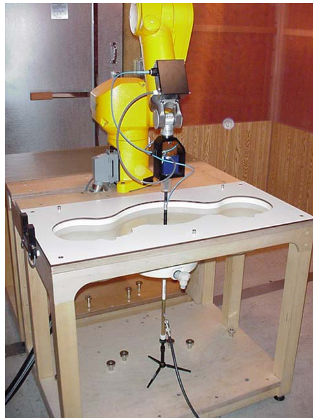
DASY4 Measurement System with SAM Phantom
