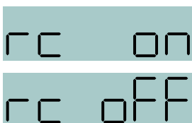
Remote Control Screens
