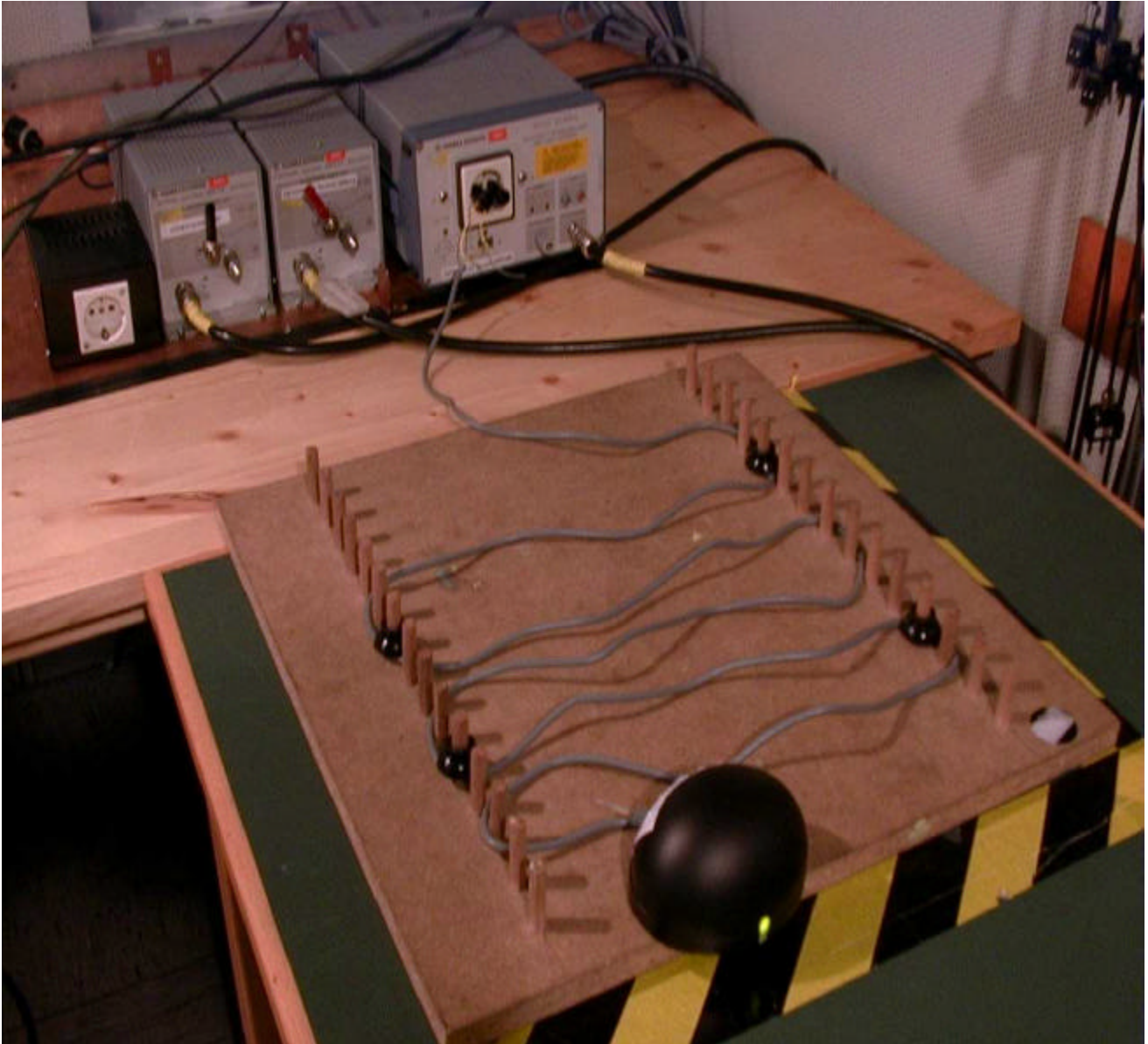
Set-up for conducted and radiated measurements <30 MHz
