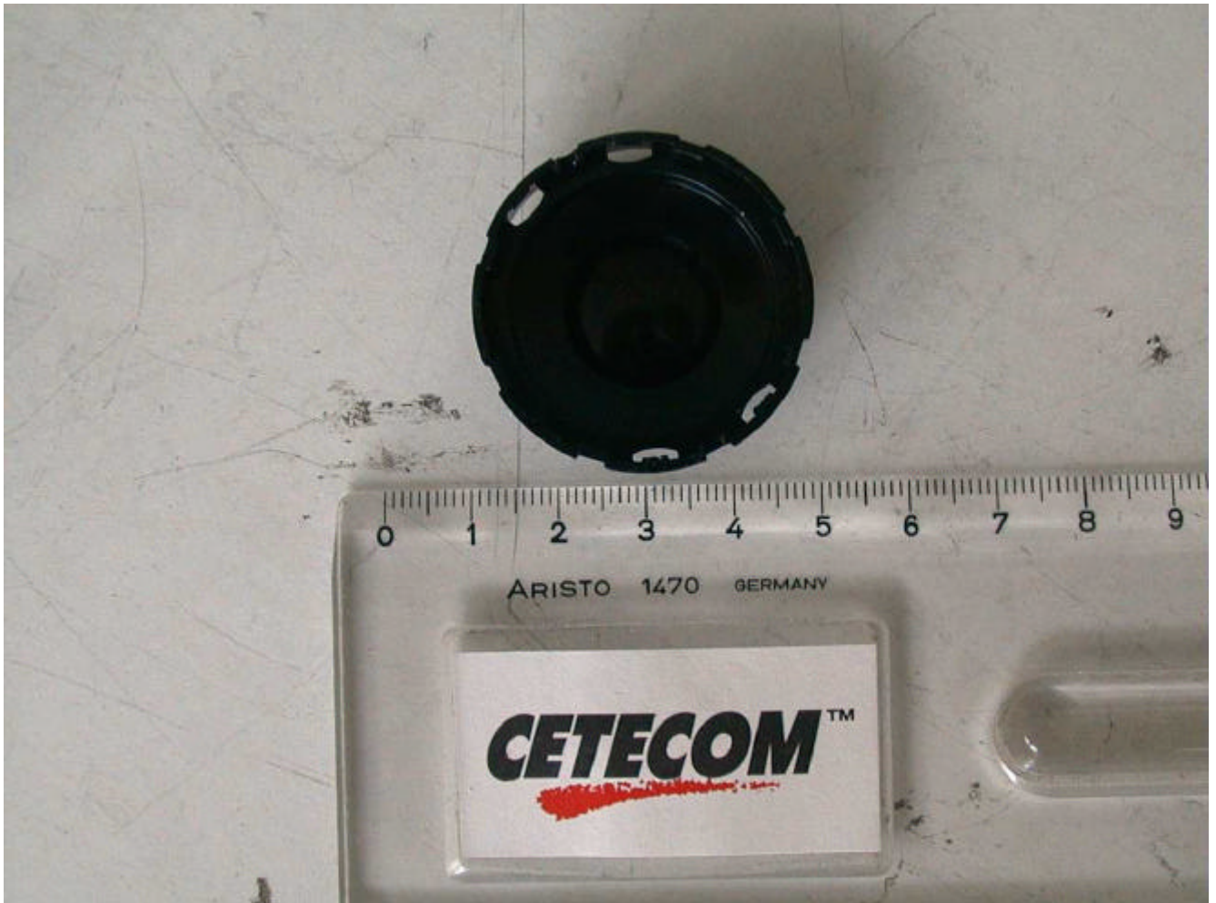
Plastic cover with dielectrical lens
