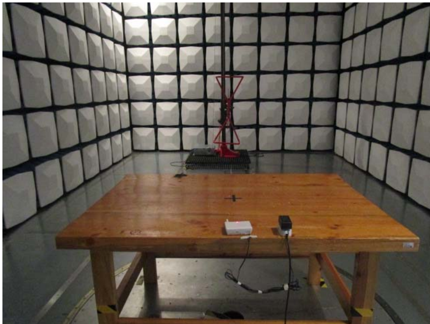
Radiated Emission –Rear View (Below 1GHz) (DC 12V)
