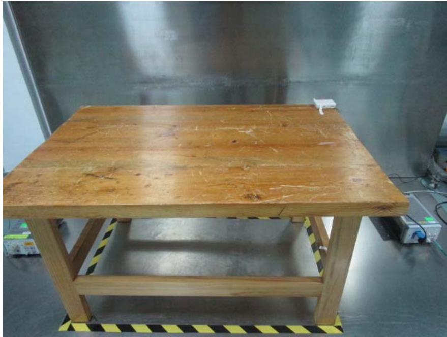
Conducted Emission--Front View (AC 12V)
