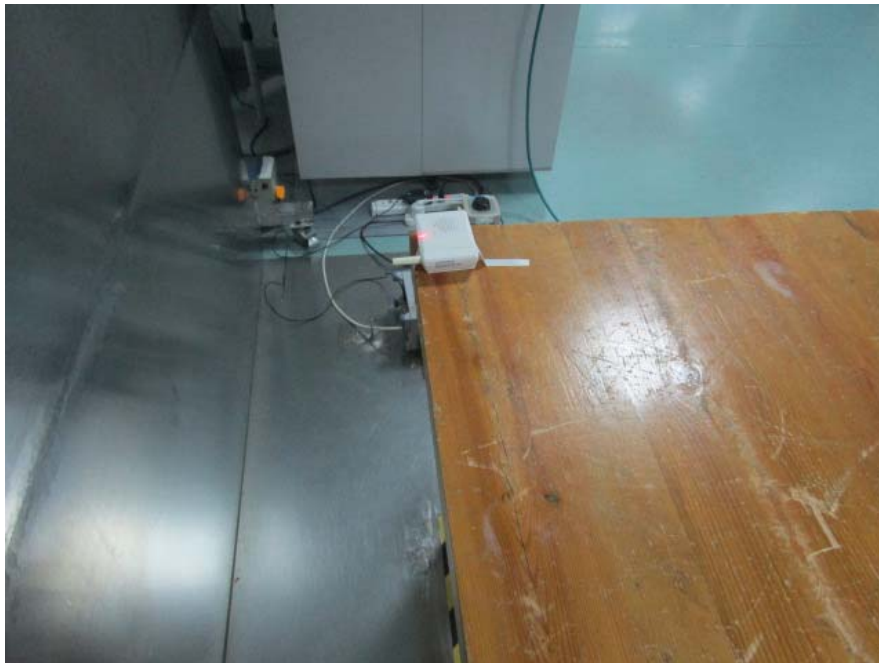
Conducted Emission – Side View (AC 12V)
