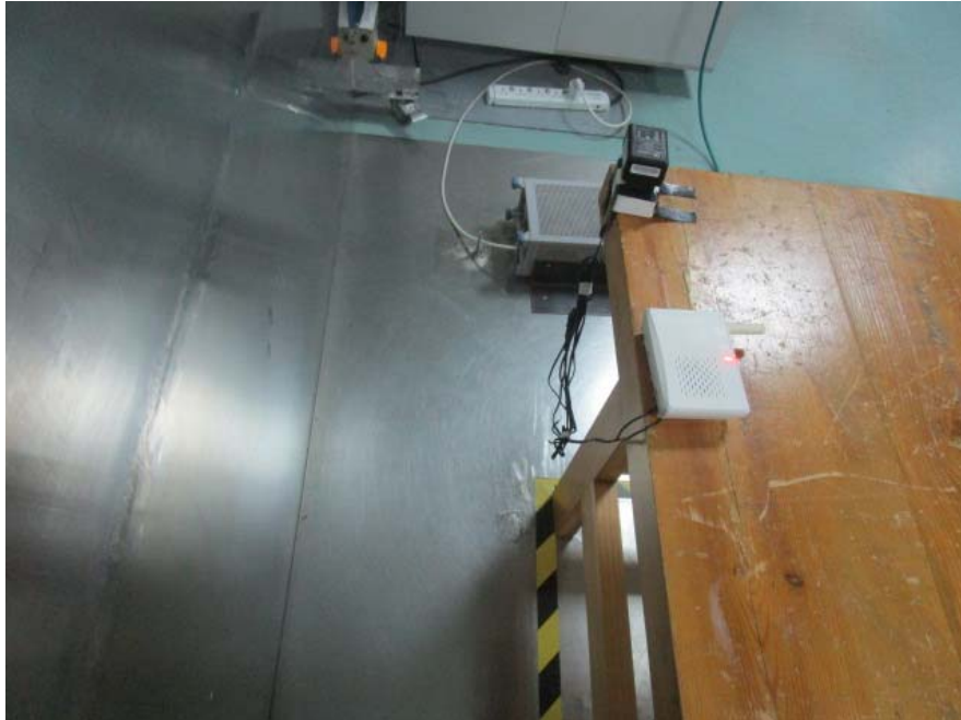
Conducted Emission – Side View (DC 12V)
