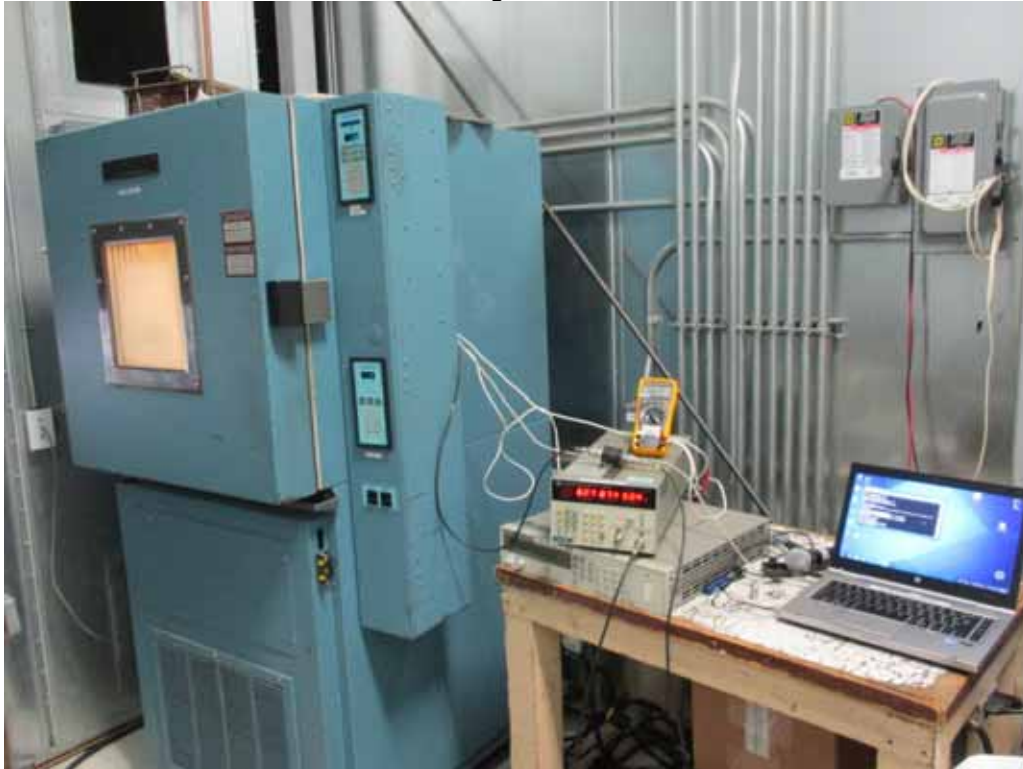
Test Setup for Frequency Tolerance Tests
