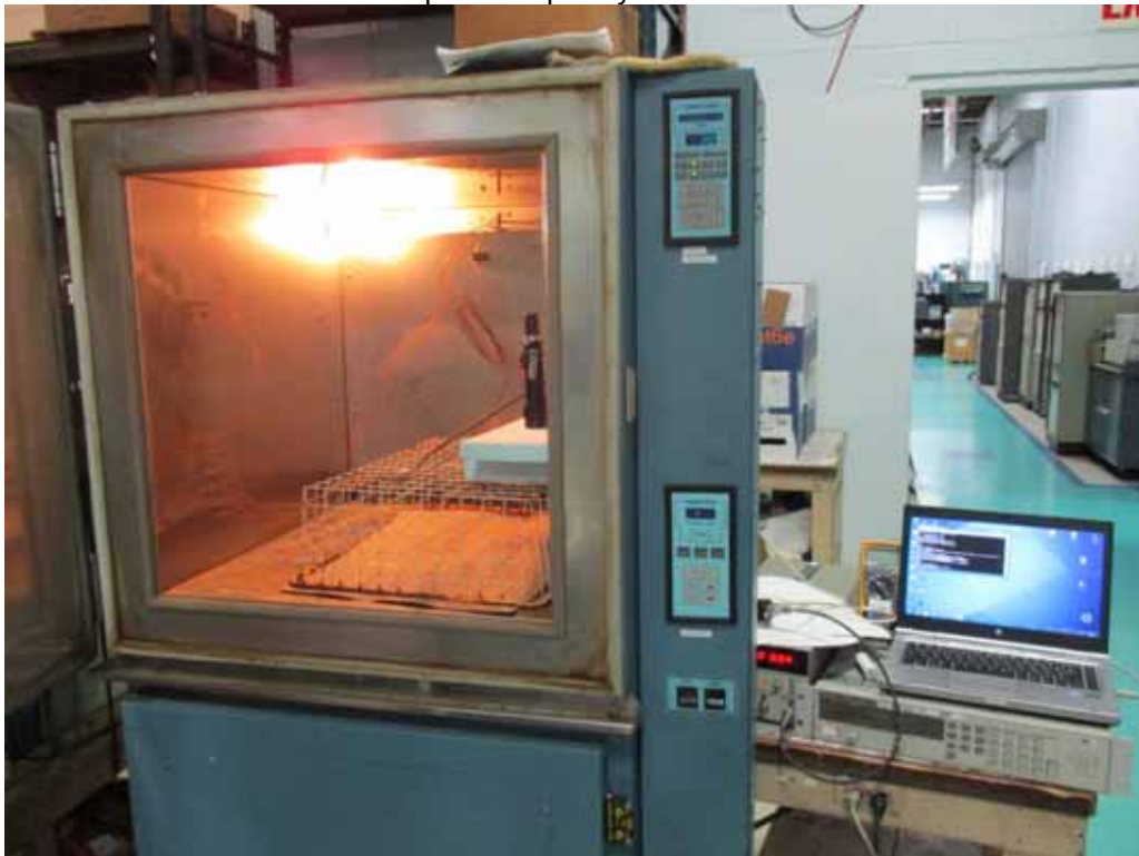
Test Setup for Frequency Tolerance Tests
