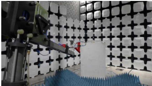
Figure 1: AXT200 Transmitter Test Setup
