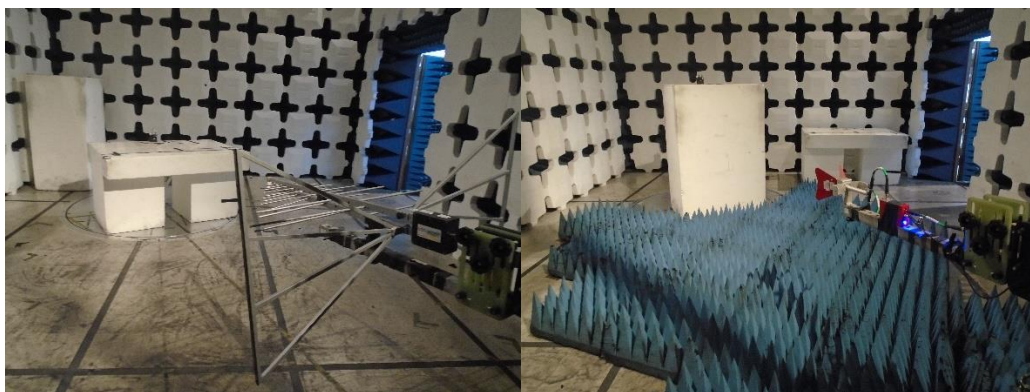
Figure B 1: QLXD1 Transmitter Test Setup
