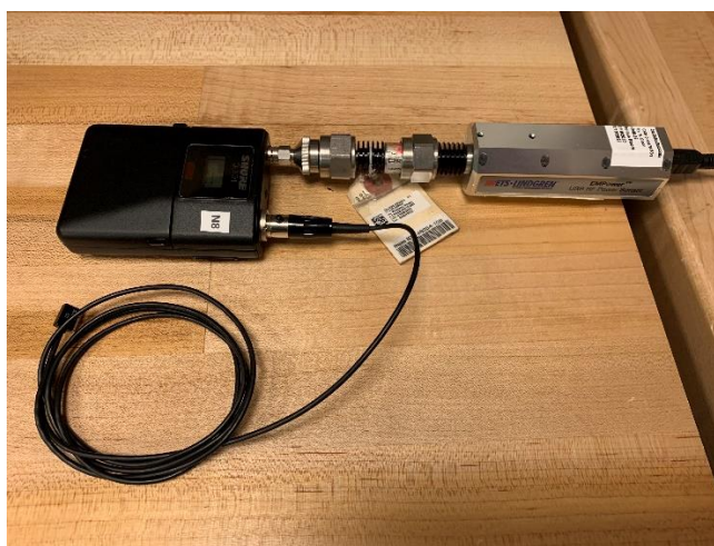
Figure C 1: Test setup for Maximum Power Output
