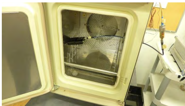
Figure D-1 - Test Setup for Frequency Stability
