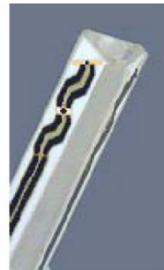
Figure 2.3 Probe Thick-Film Technique
