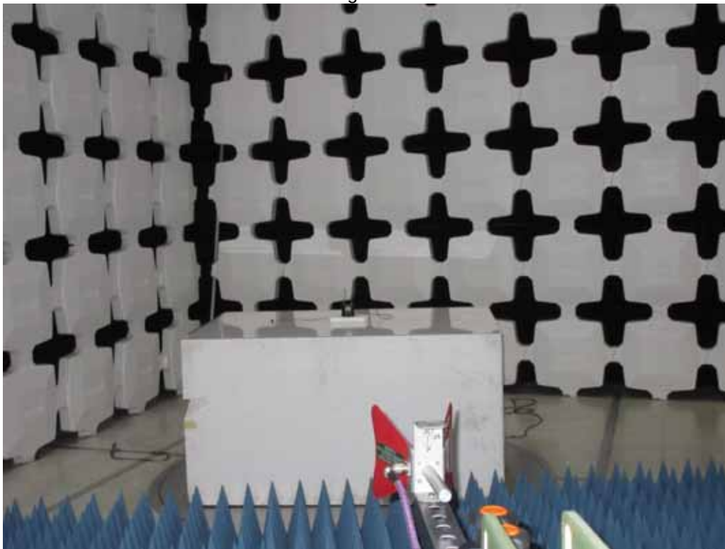
Test Setup for Radiated Emissions, 1GHz to 10GHz – Horizontal Polarization
