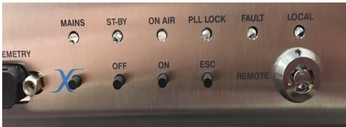
Close up view of indicator lights
