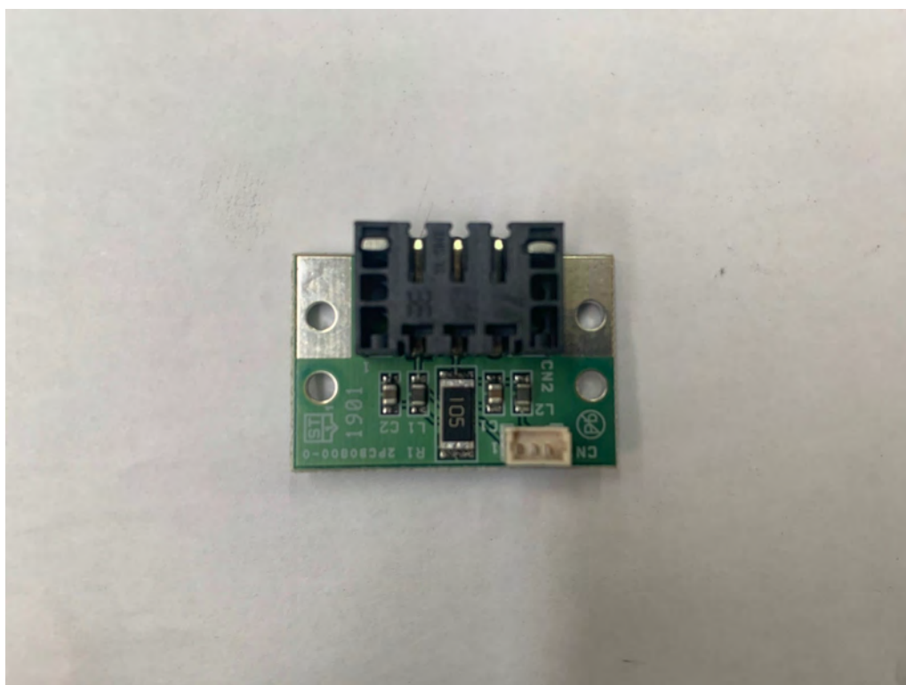
TG5K8A884-0 SEPARATE INTERLOCK BOARD TOP
