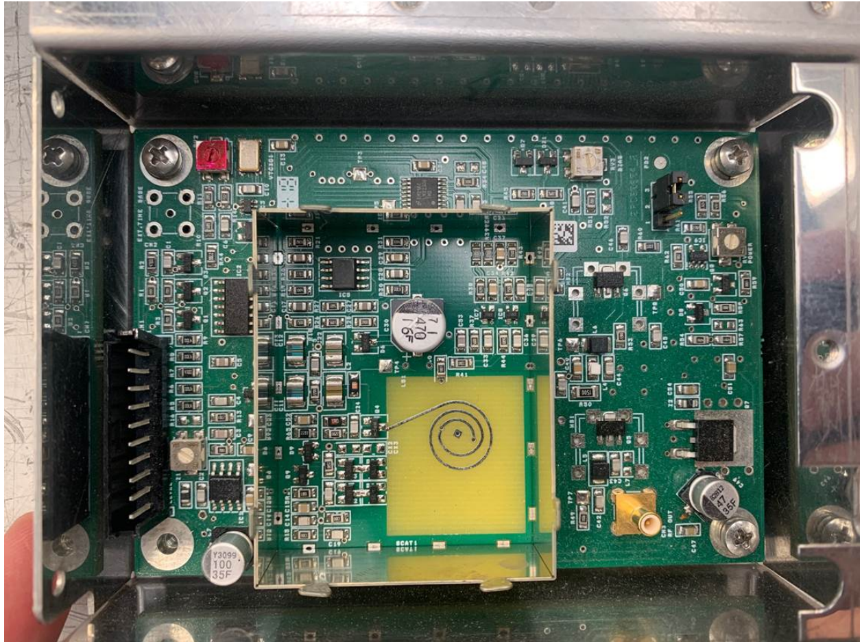
VCO BOARD – TOP VIEW – SHIELD REMOVED
