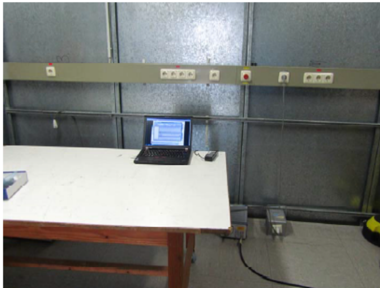
Test setup for radiated emission measurement 9 kHz – 30 MHz
