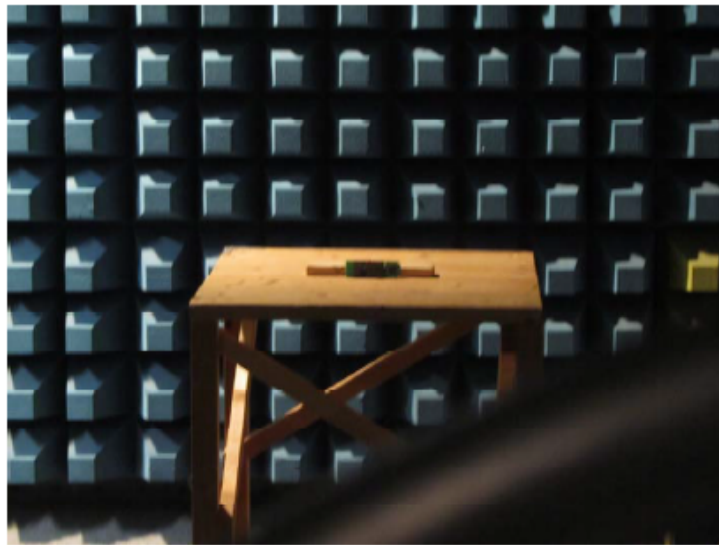
Test setup for radiated emission measurement (fully anechoic room)
