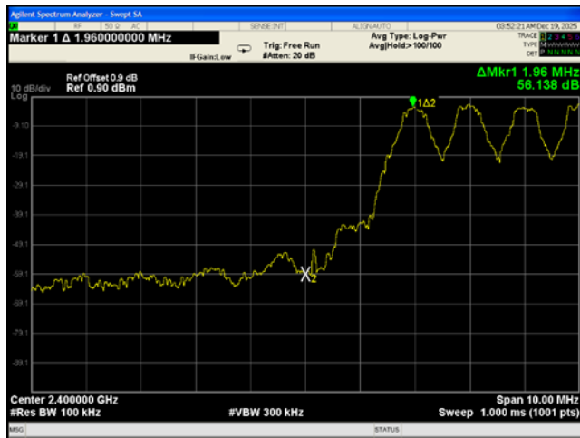
Band Edge – DH5 Low Channel Center Freq. 2.400GHz (BT with Hopping Enabled)
