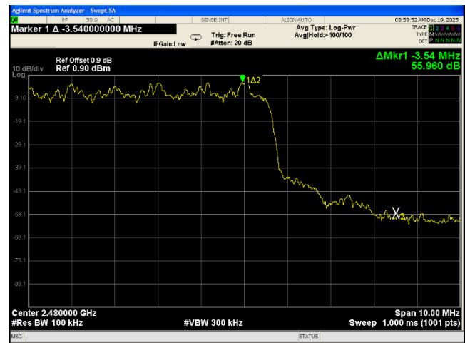
Band Edge – 3DH5 High Channel Center Freq. 2.4835GHz (BT with Hopping Enabled)
