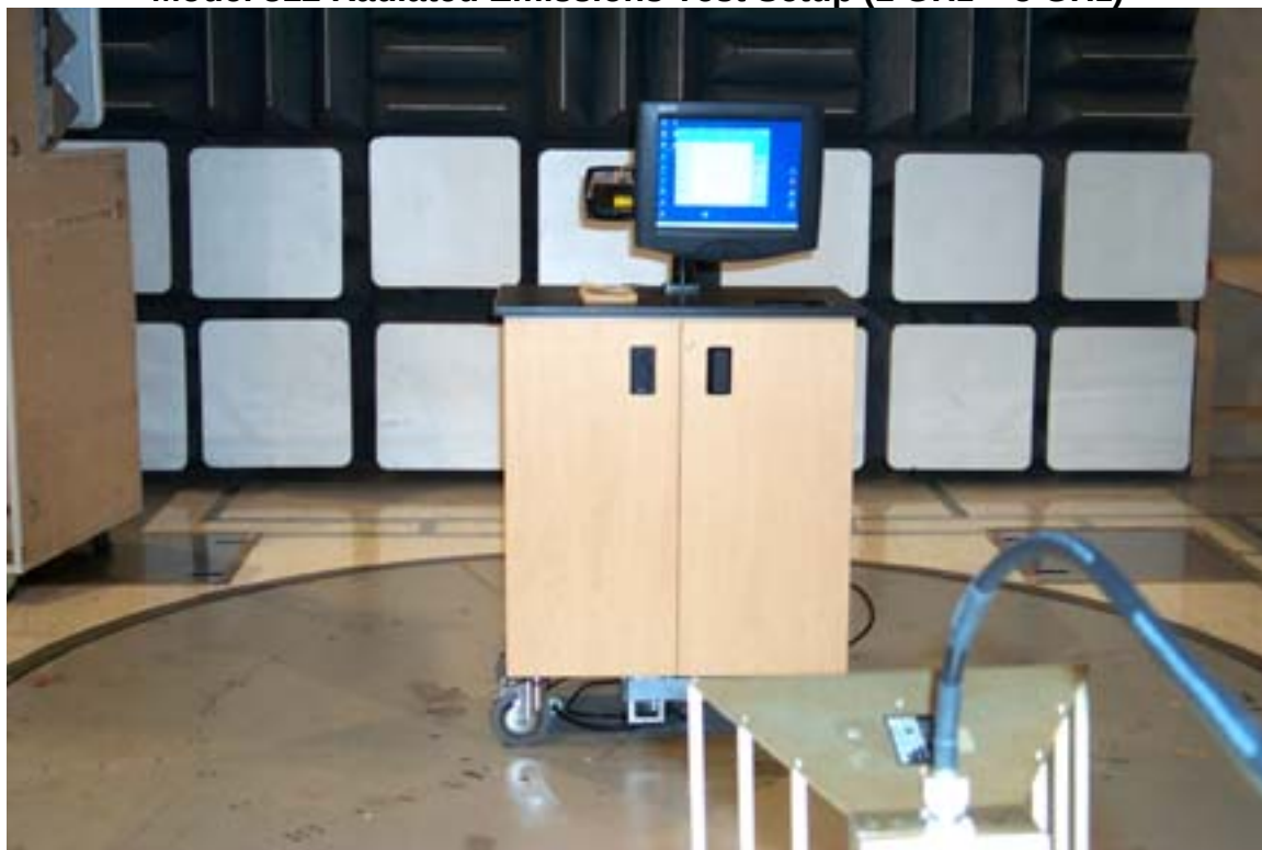
Model 812 Radiated Emissions Test Setup (1 GHz – 5 GHz)
