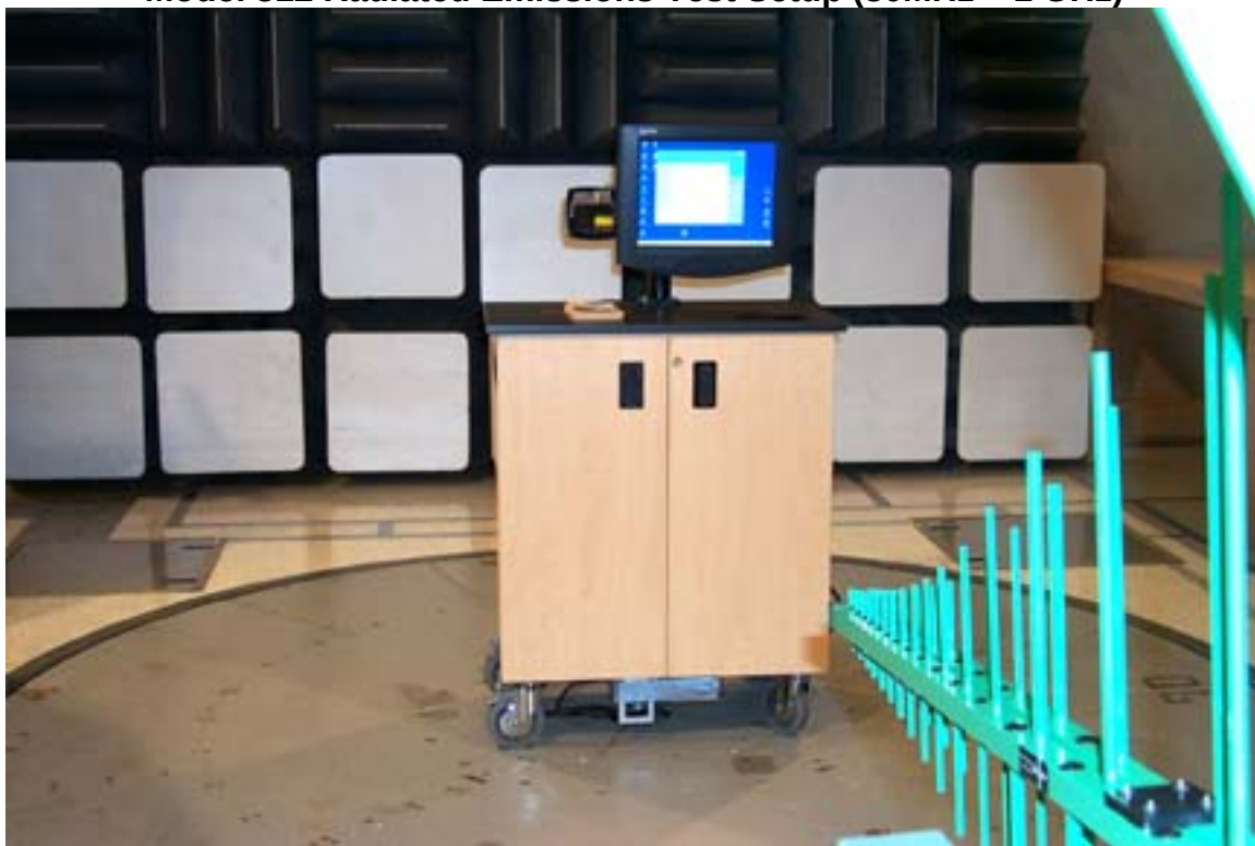
Model 812 Radiated Emissions Test Setup (80MHz – 1 GHz)
