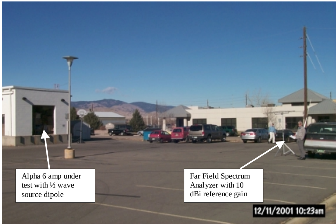
Figure 3.4.1-1 Far field test set-up
