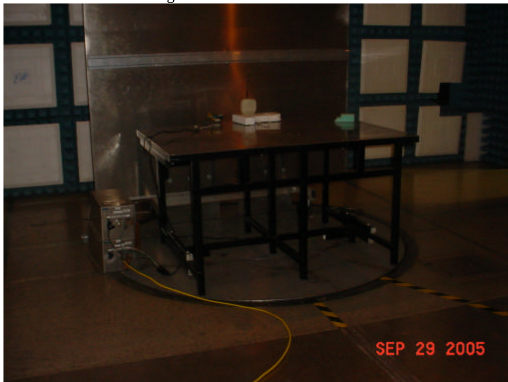
Test Setup for Conducted Emissions – P4243ME
