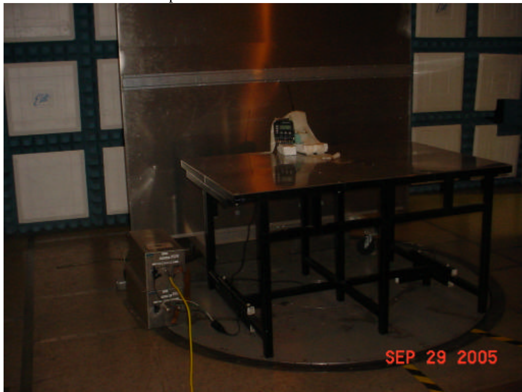
Test Setup for Conducted Emissions – P1353ME
