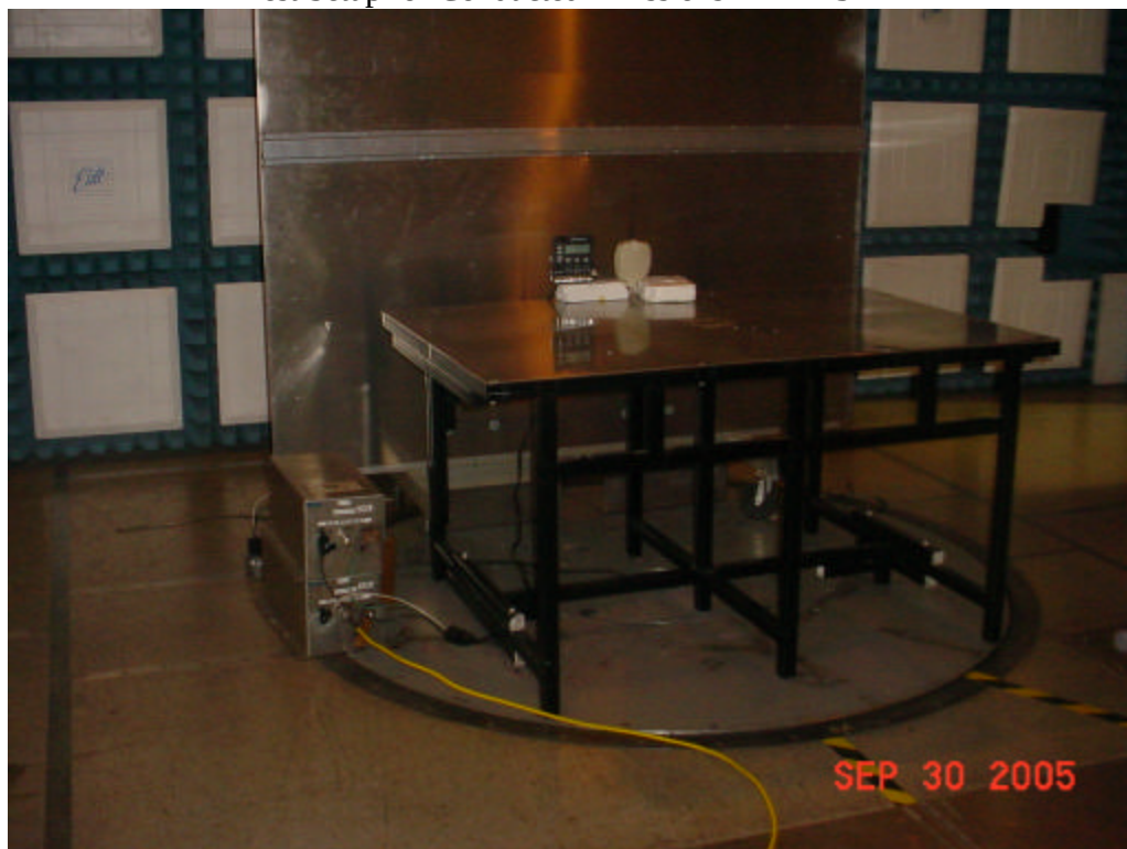
Test Setup for Conducted Emissions – P1353ME
