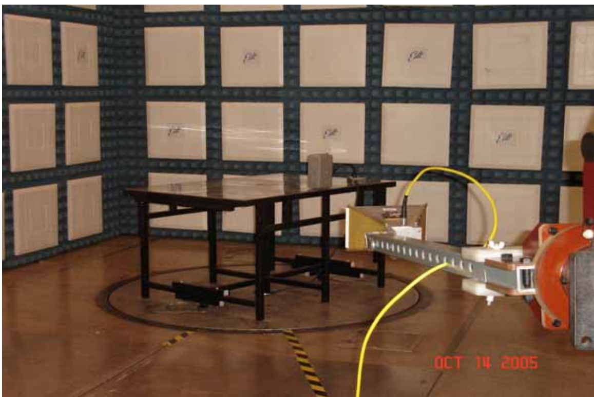
Test Set-up for Radiated Emissions, 908.3MHz – Vertical Polarization
