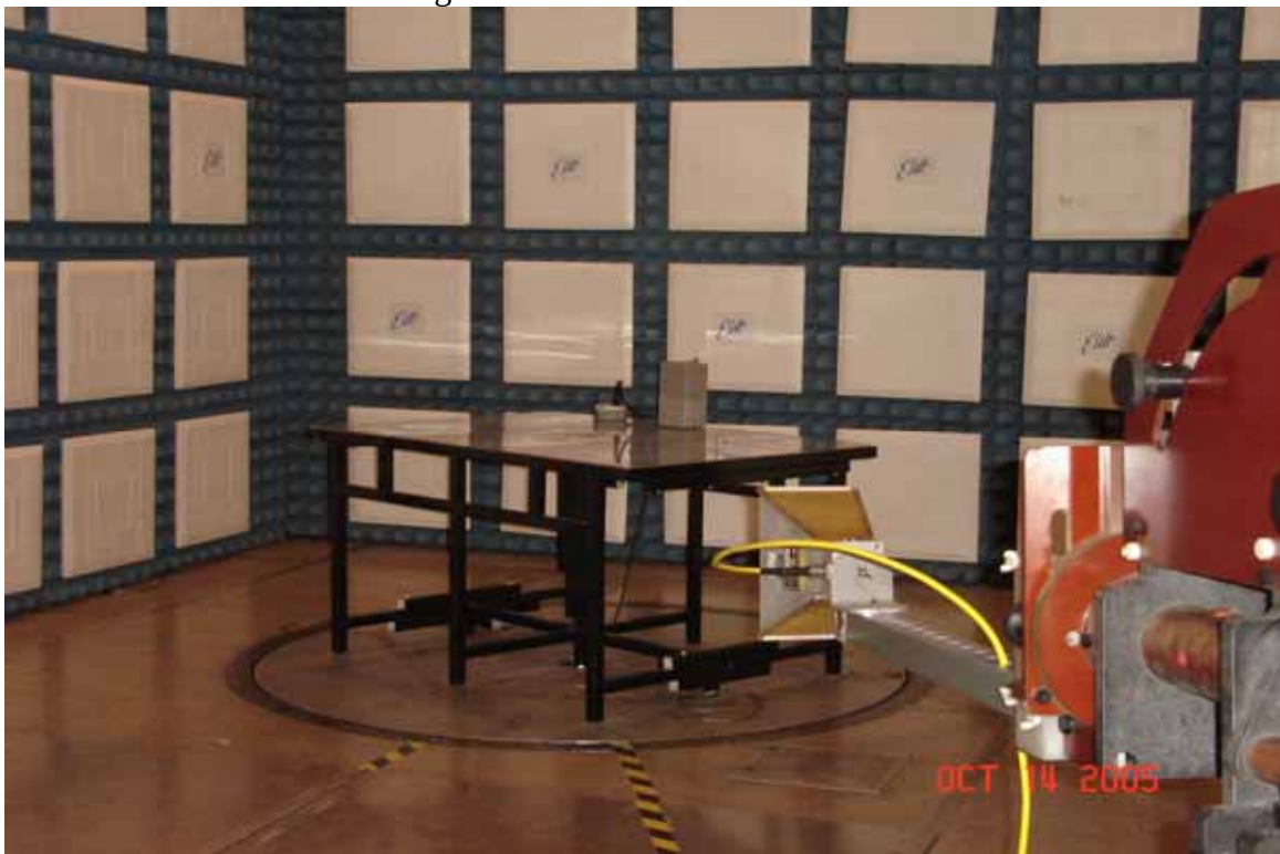
Test Set-up for Radiated Emissions, 1GHz to 5GHz – Horizontal Polarization
