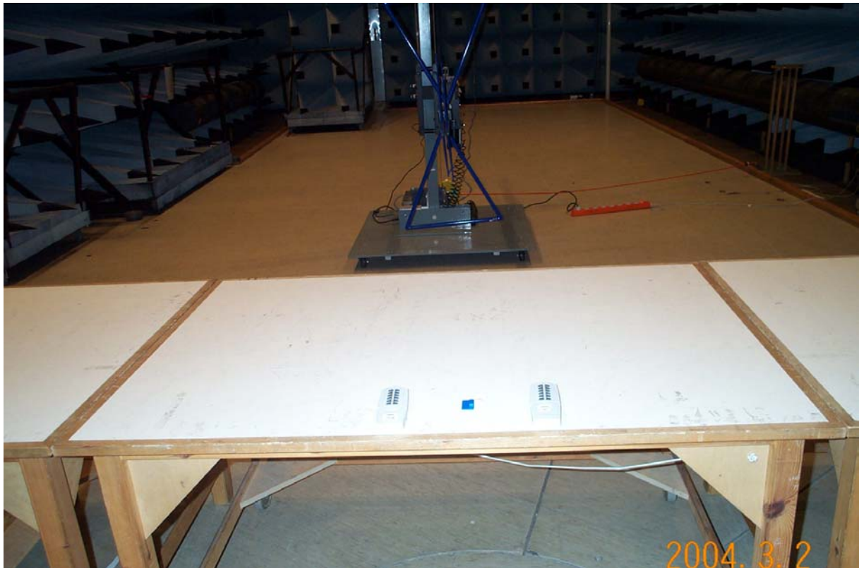
Photo 1 Set-up for measurements 30 - 1000 MHz. Date is correctly 2004-02-13.
