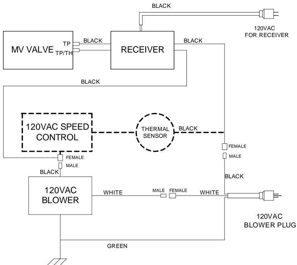
Connect the two 30” long 18AWG wires labeled “110VAC FAN ONLY” between receiver and blower as shown in the following diagram as well.
