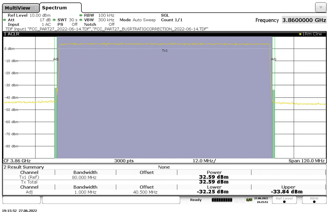
Figure 231: Out-of-Band Emission, 1cc-3 (OBW=80MHz), High Channel, 256QAM_TM3.1a, TX Port 17
