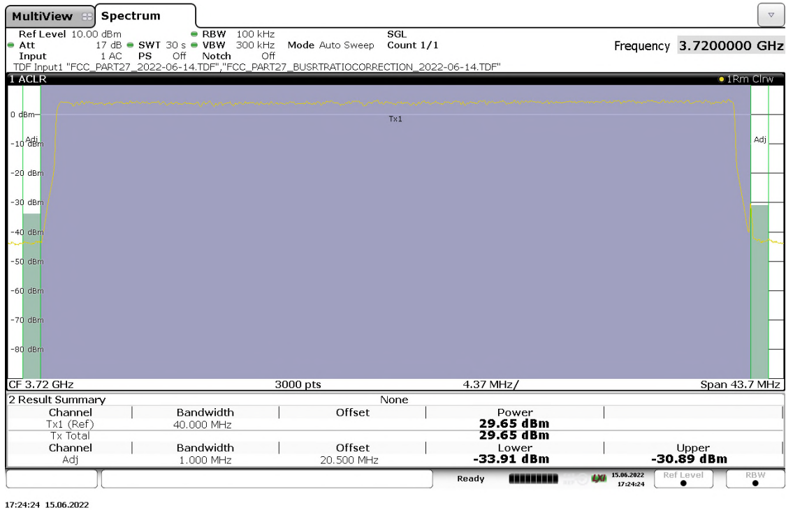
Figure 226: Out-of-Band Emission, 1cc-1 (OBW=40MHz), Low Channel, 256QAM_TM3.1a, TX Port 28
