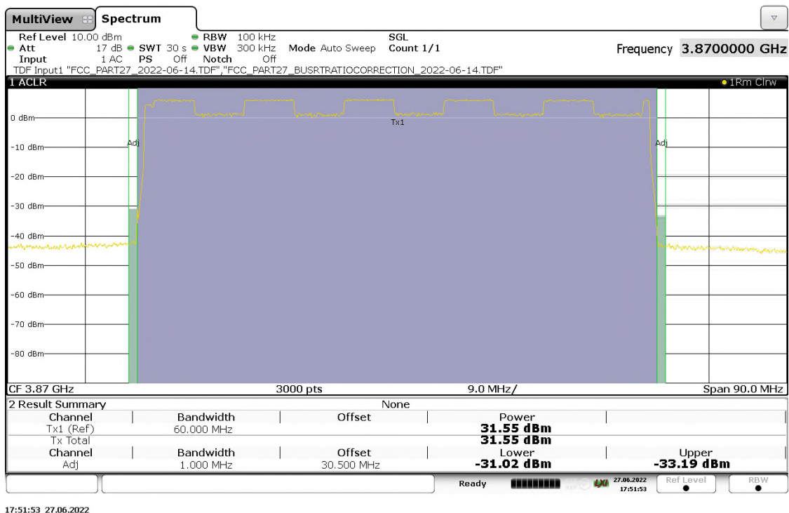
Figure 229: Out-of-Band Emission, 1cc-2 (OBW=60MHz), High Channel, 16QAM_TM3.2, TX Port 17
