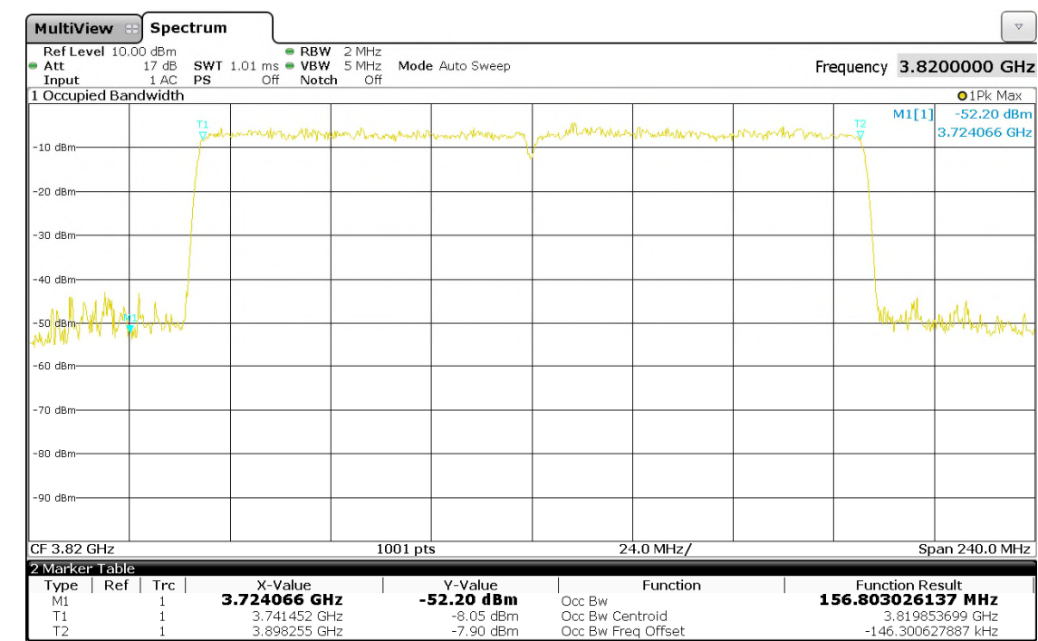
Figure 217: 99% Occupied Bandwidth, 2cc-3a (OBW=80MHz+80MHz), 256QAM_TM3.1a, High Channel, TX Port 25
