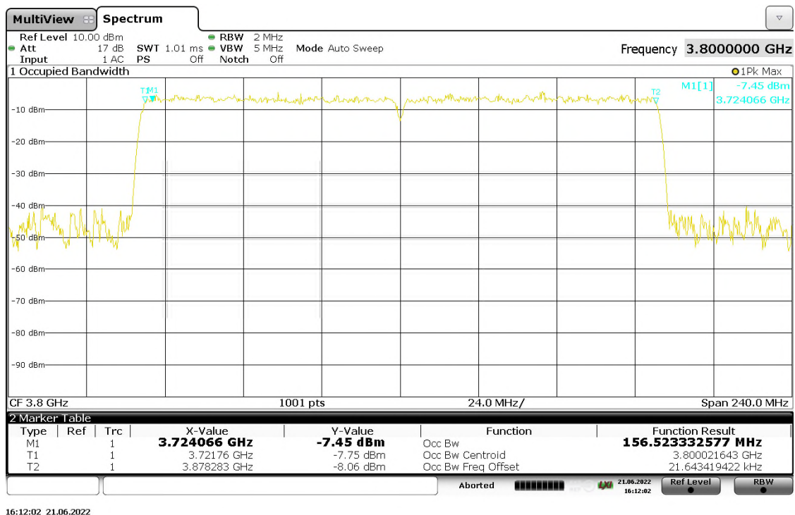
Figure 207: 99% Occupied Bandwidth, 2cc-3a (OBW=80MHz+80MHz), 64QAM_TM3.1, Middle Channel, TX Port 31
