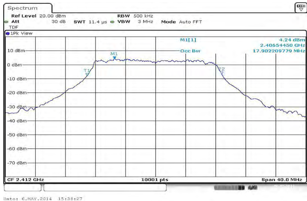
Plot 1: TX mode, lowest channel
