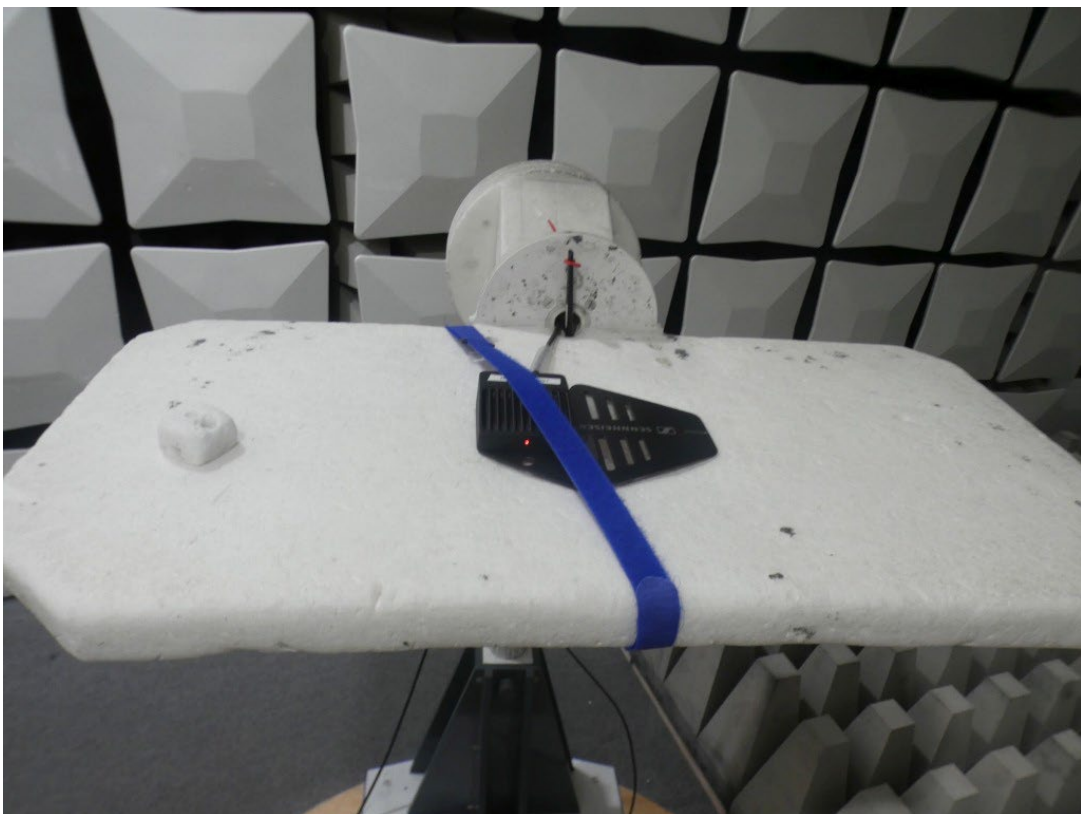
Photo 4: Setup Spurious Emissions Radiated (FAC), > 1GH, detail view
