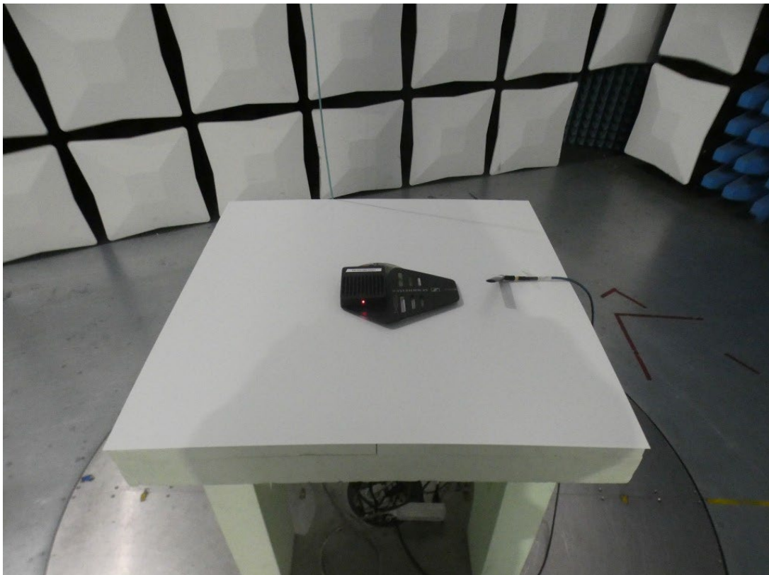
Photo 2: Setup Spurious Emissions Radiated (SAC), < 1 GHz, detail view
