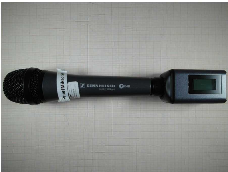
Photo 8: microphone with RF part
