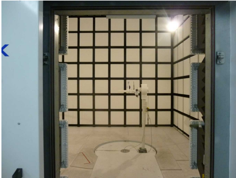
Photo 1: EUT at the anechoic chamber
