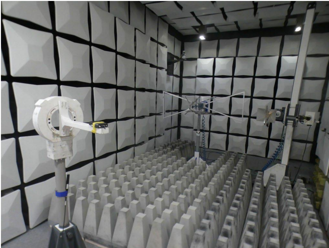
Photo 3: Setup Spurious Emissions Radiated (FAC), > 1GHz
