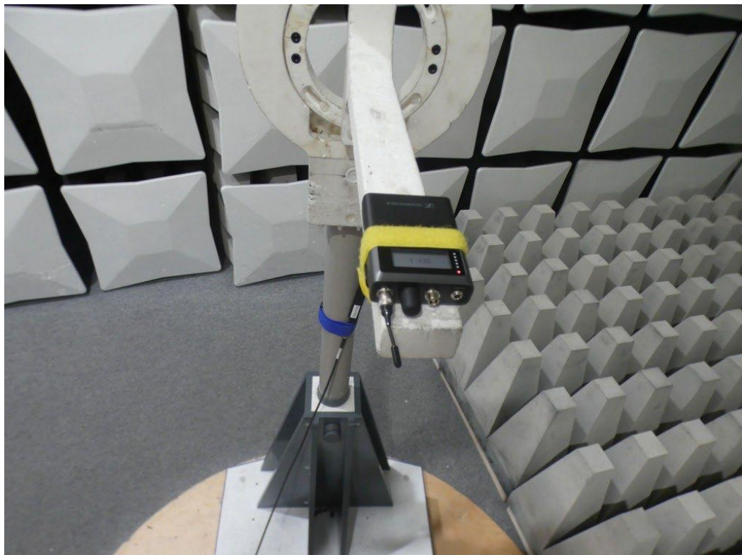
Photo 4: Setup Spurious Emissions Radiated (FAC), > 1GHz, detail view
