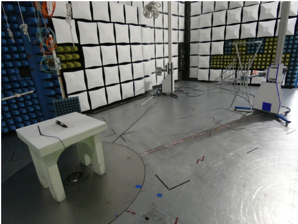
Photo 1: Setup Spurious Emissions Radiated (SAC), < 1 GHz, EUT horizontal
