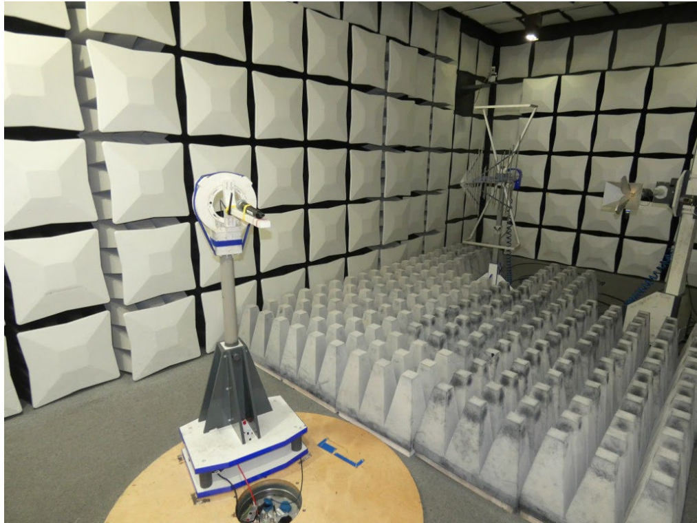
Photo 5: Setup Spurious Emissions Radiated (FAC), > 1GHz
