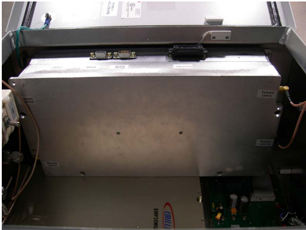
Figure 3: Internal – Assembled View - Channelizer
