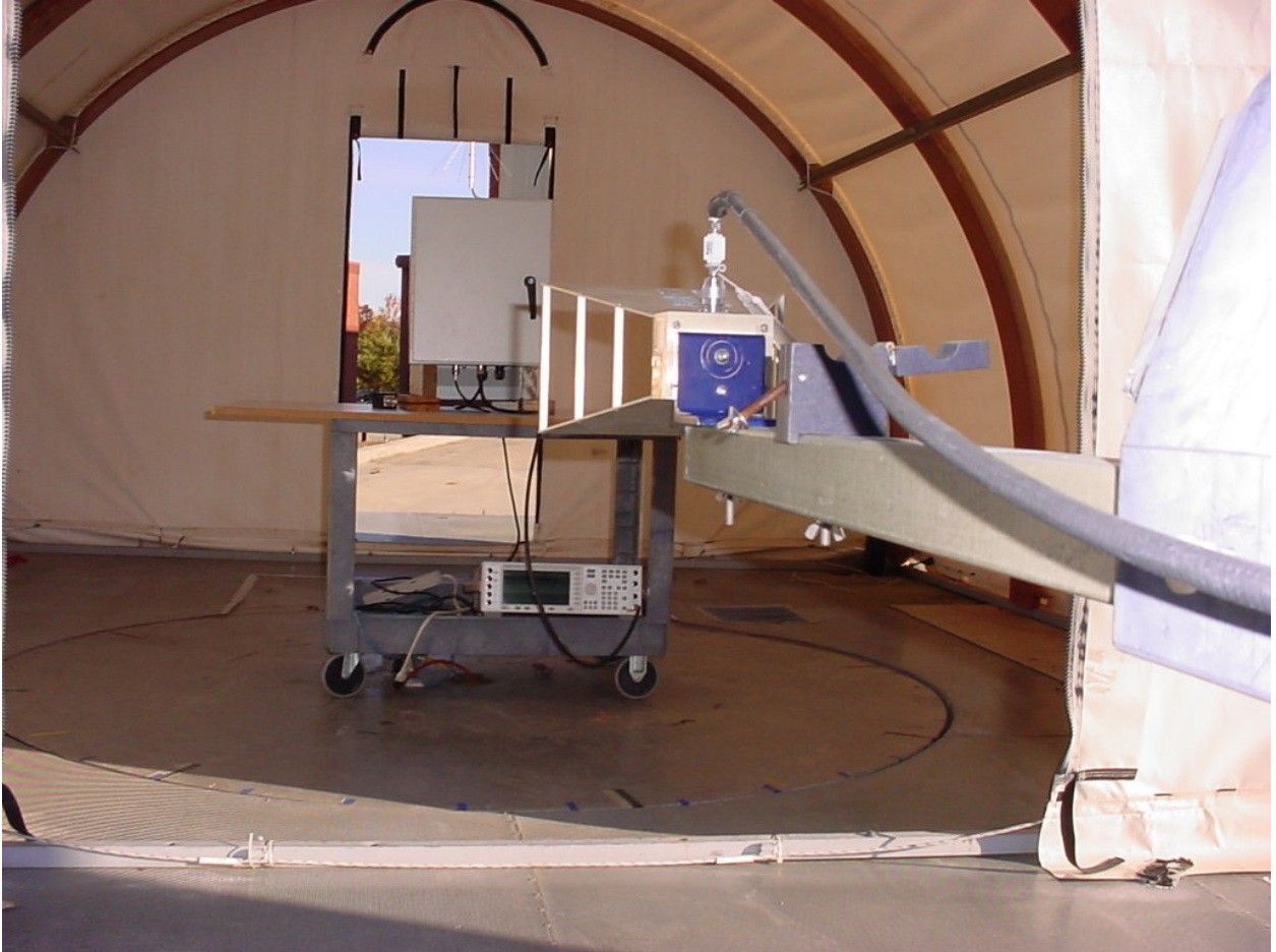
Figure 2: Test Setup - Radiated Emissions - Intentional
