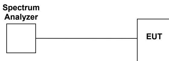
Figure 6.4.1-1: Occupied Bandwidth Test Setup
