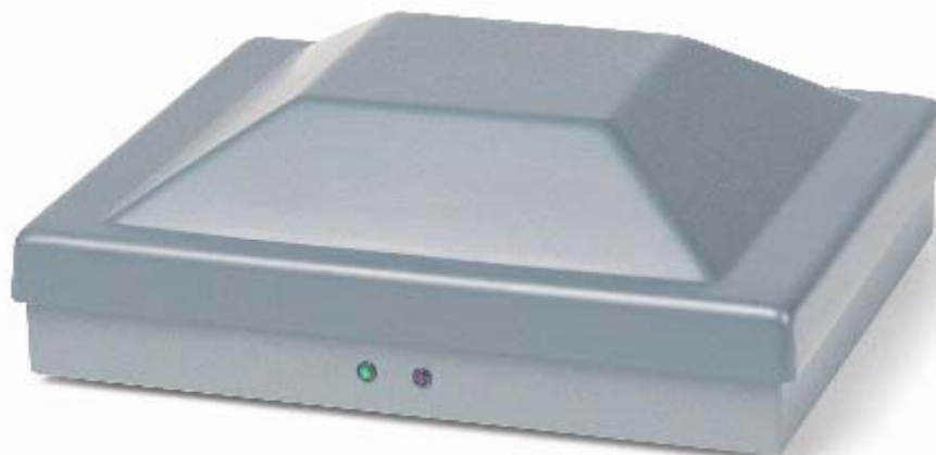
Figure 1.13 Circulation Circuit Programmer
