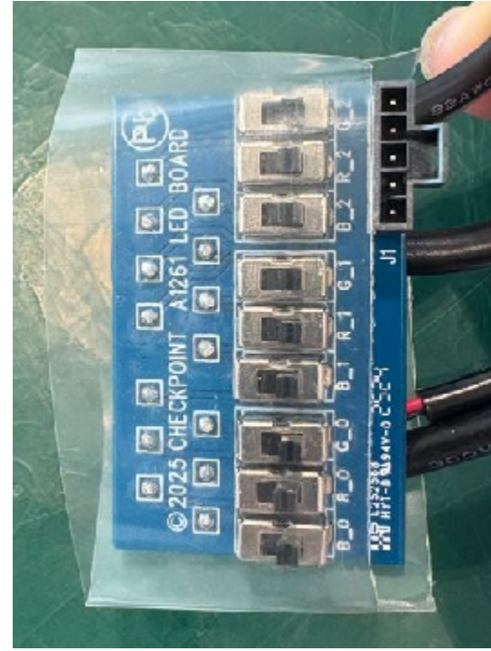
3. COVER LED SELECTOR BOARD WITH THE TUBE
