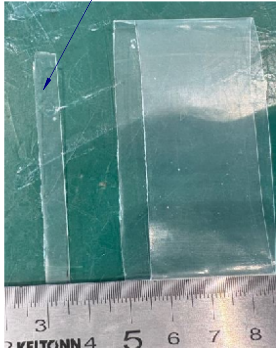
2. ADD A CUT OF 5mm TO THE HEAT SHRINK TUBE
