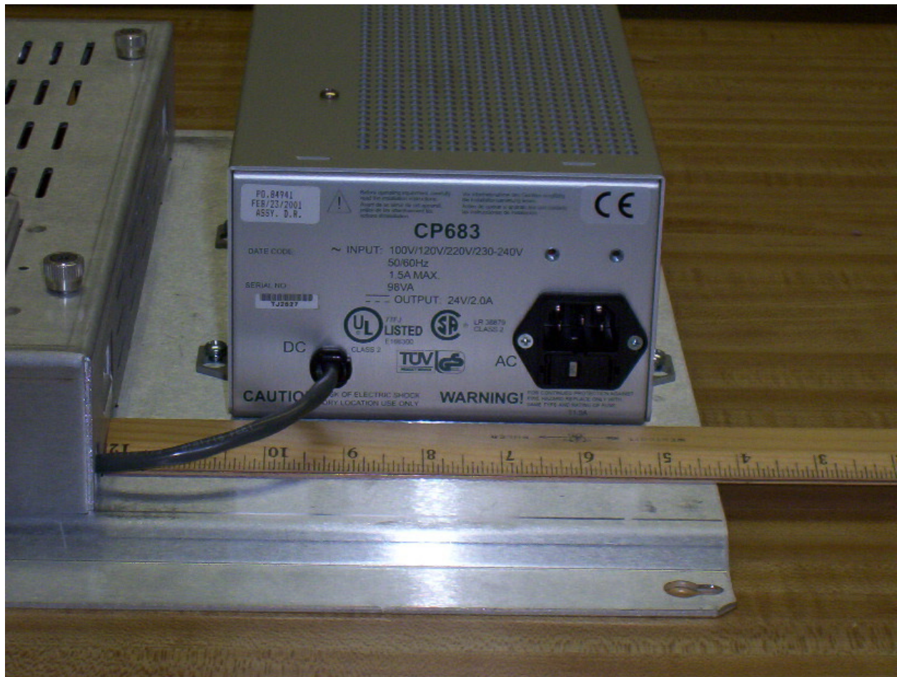
Photo 4 – Power Supply Labeling Information
