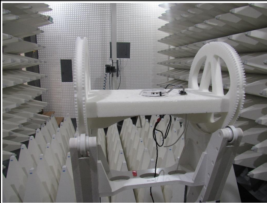
Setup for measurements above 1 GHz (EUT Side)
