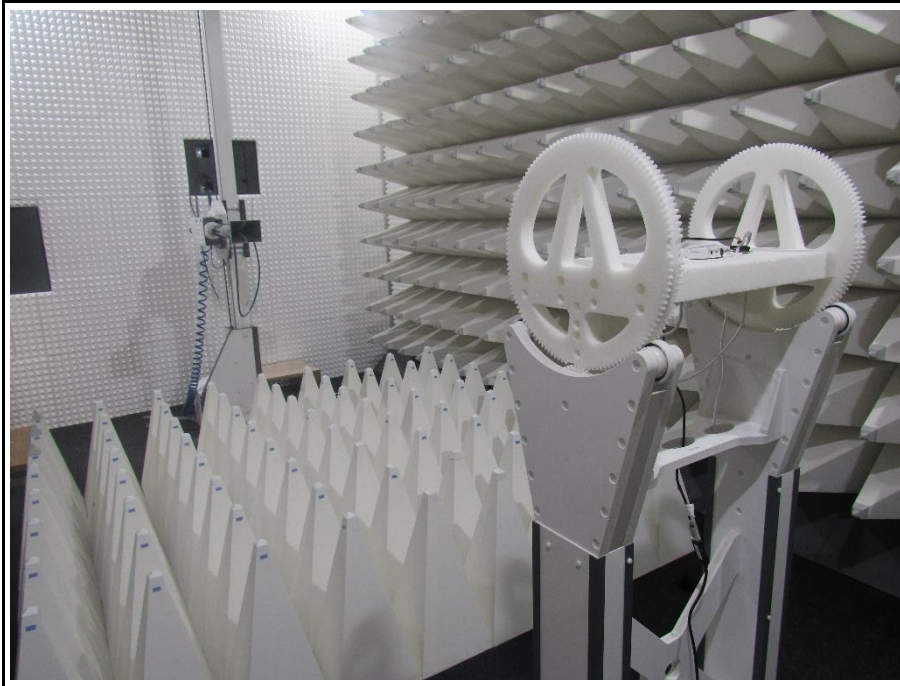
Setup for measurements above 1 GHz (EUT Side)
