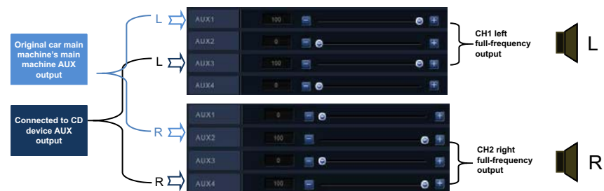
Example 3: Illustration of original car main machine's AUX connected to CD device, AUX mixing input and stereoscopic full-frequency output
