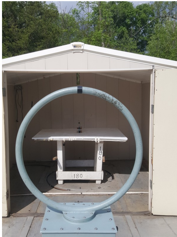
Figure 3.1 Radiated Test Setup
