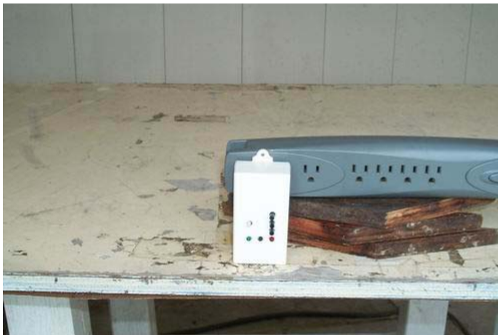
Figure 3.1 Radiated Test Setup, position 1-X
