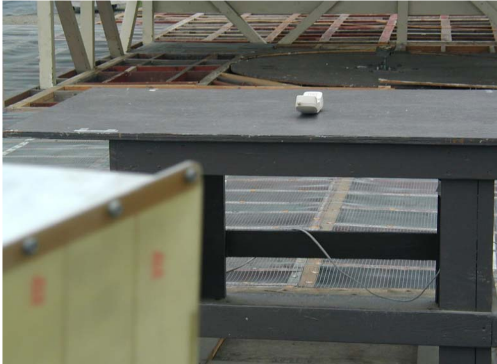
Figure 3: Band-Edge and 6dB Test Set-up Photo for Headset Unit (Front View)
