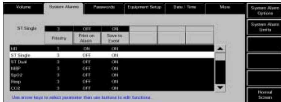
FIGURE 9-7 System Alarms (Alarm Responses) Tab
