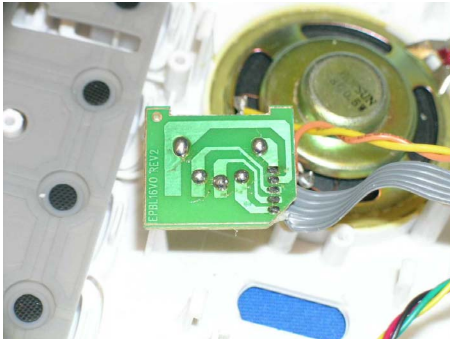
Corded Phone's Headset Volume Control solder side
