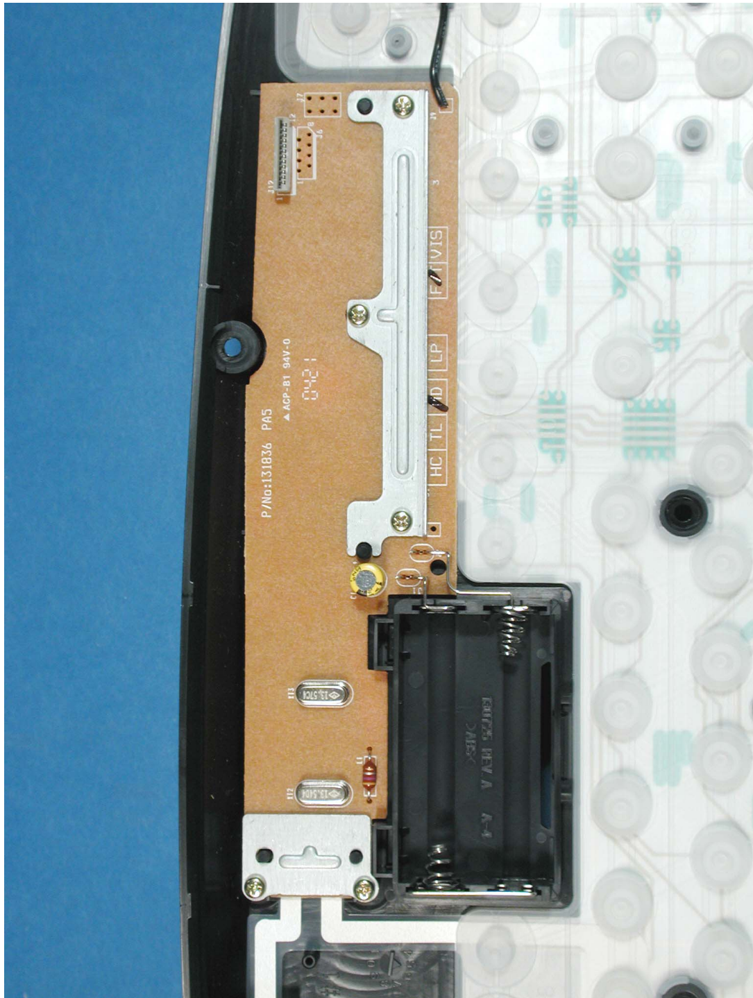
Photograph 2: Y-RR54 internal view (RF part)
