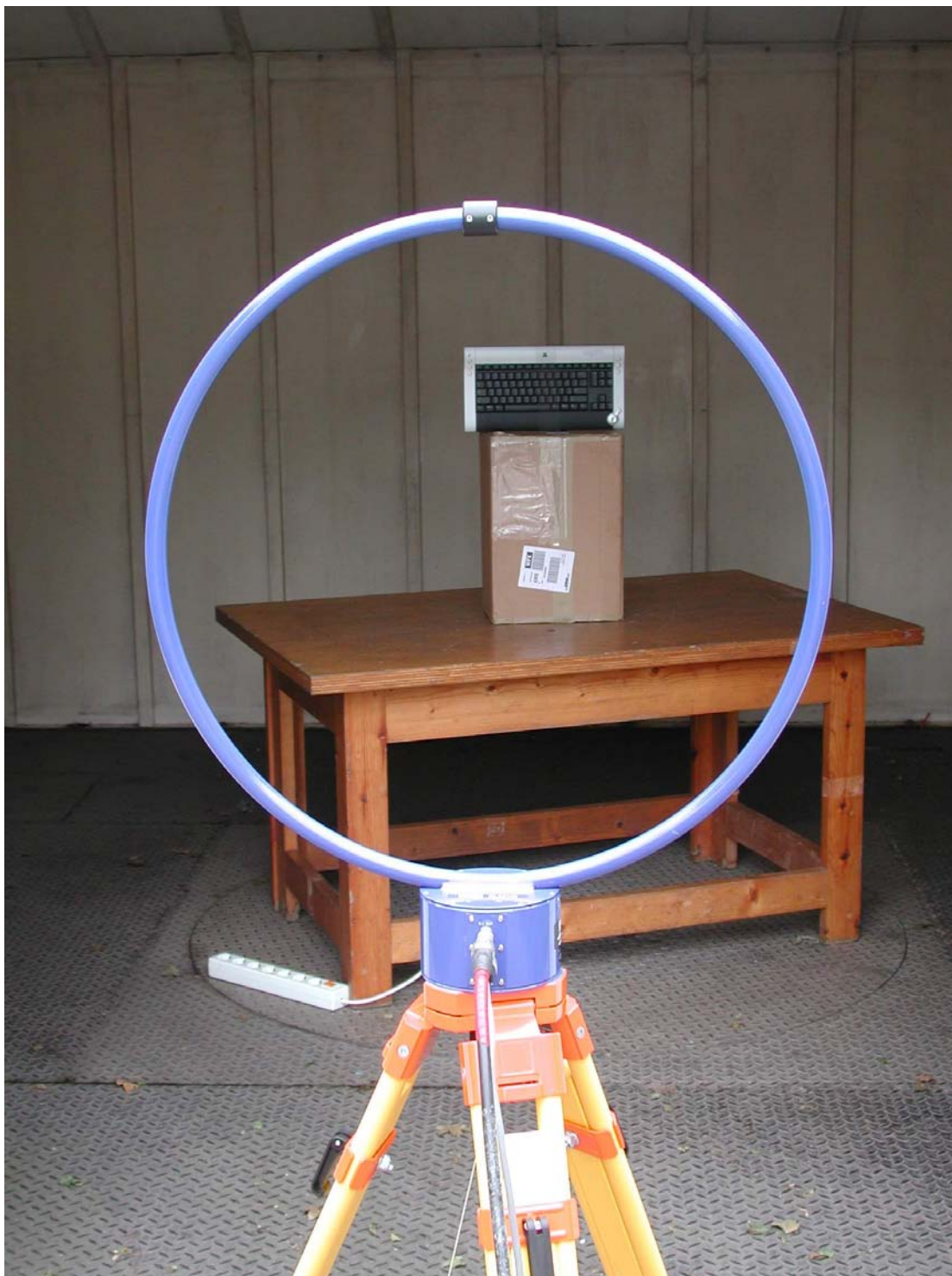
EUT on turn table in X-position
