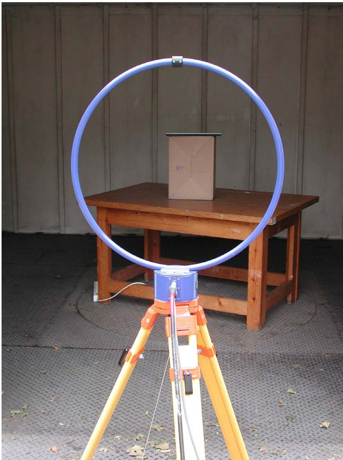
EUT on turntable in Y-position
