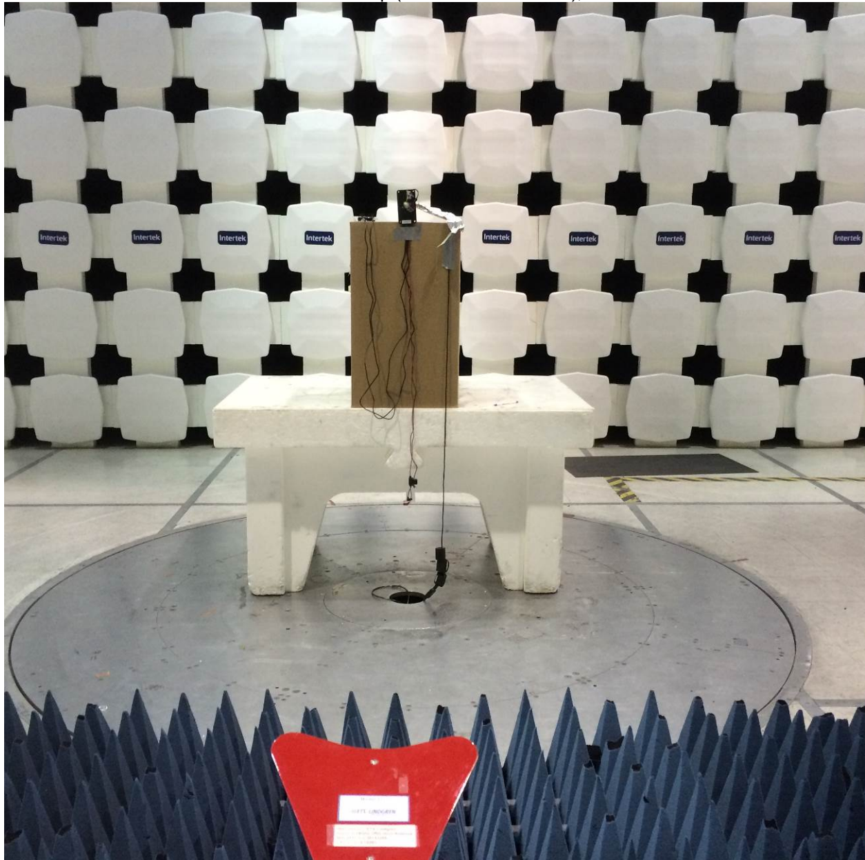
1-18 GHz Test Setup (EUT on its short side), Photo 1
