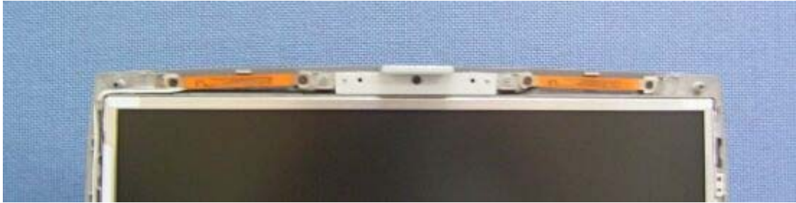
Picture of Antenna installed in the notebook
