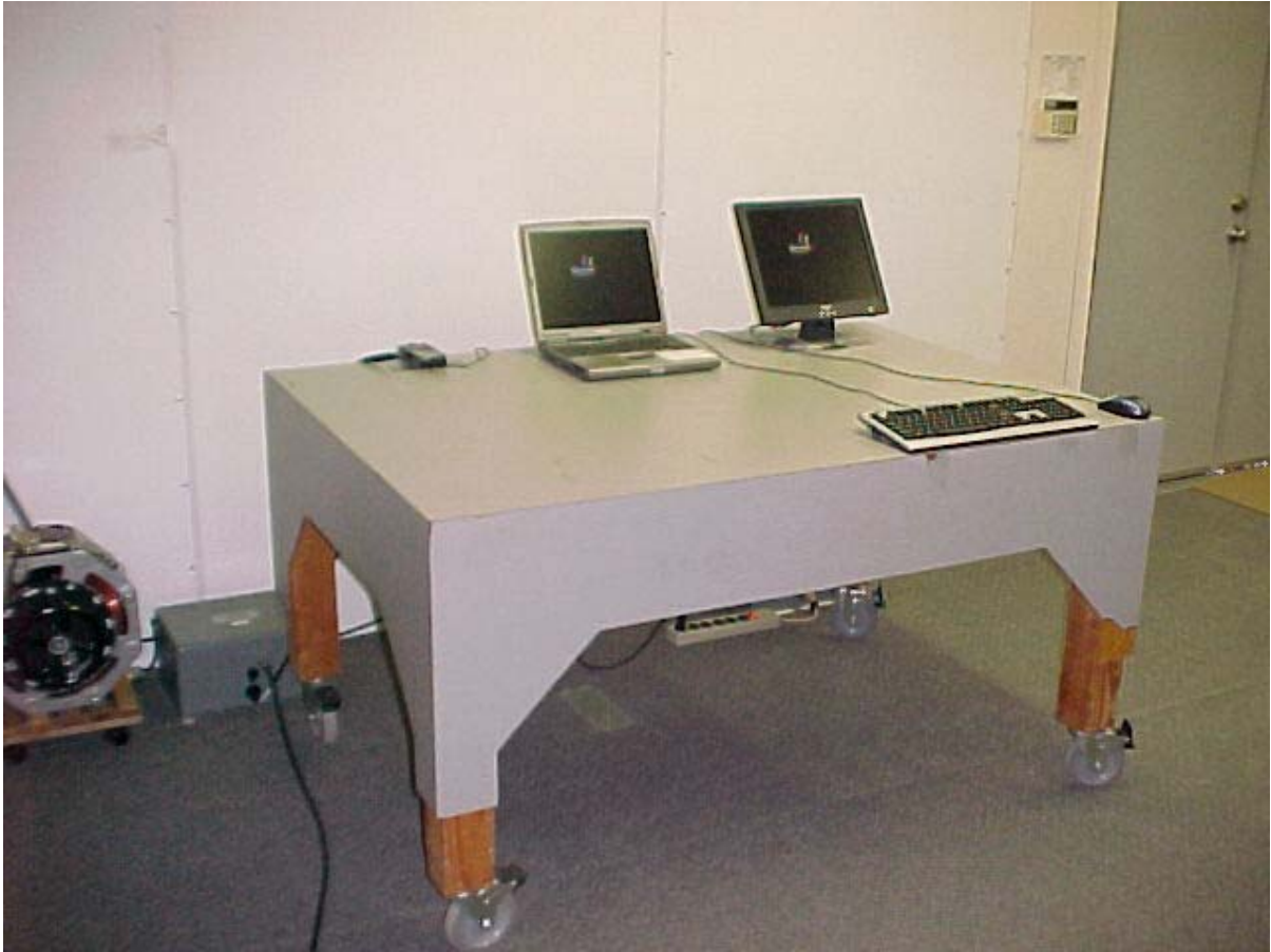
AC Conducted Emissions Measurement (Front View) Setup
